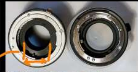
Left: Variable tube, diameter too small, vignettes Right: normal tube, larger diameter
